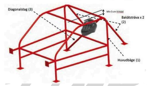
**11.9.1** Dimensions for protective cage: For main arch, possibly longitudinal main arch, diagonal bracing applies 45mm diameter x 2.5 mm or 50mm x 2 mm) material thickness and for other pipes; 38mm diameter x 2.5 mm material thickness or 40 x 2.0 mm. All pipes must consist of cold drawn seamless unalloyed steel pipe, containing a maximum of 0.3% carbon and with a minimum yield strength of 350 N/mm2. **11.9.2** Attachment points for protective cage:
