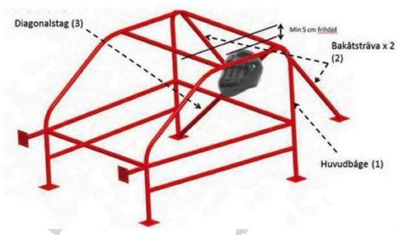
**11.8** Dimensions for protective arch/protective cage: For main arch, possibly longitudinal main arch, diagonal brace applies 45mm diameter x 2.5 mm or 50mm x 2 mm) material thickness and for other pipes; 38 mm diameter x 2.5 mm material thickness or 40 x 2.0 mm. All pipes must consist of cold-drawn seamless unalloyed steel pipes, containing a maximum of 0.3% carbon and with a minimum yield strength of 350 N/mm2.
