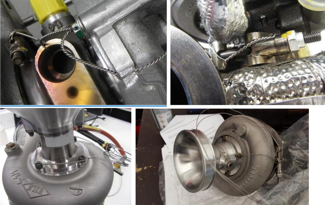
Examples of incorrect sealing wiring
